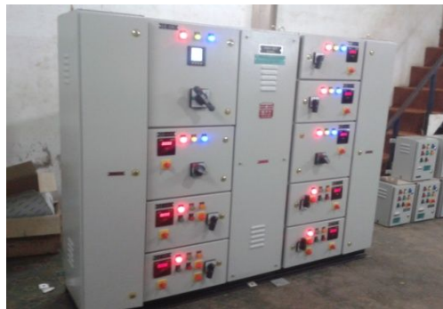
Air Cool chillers Control Panel
